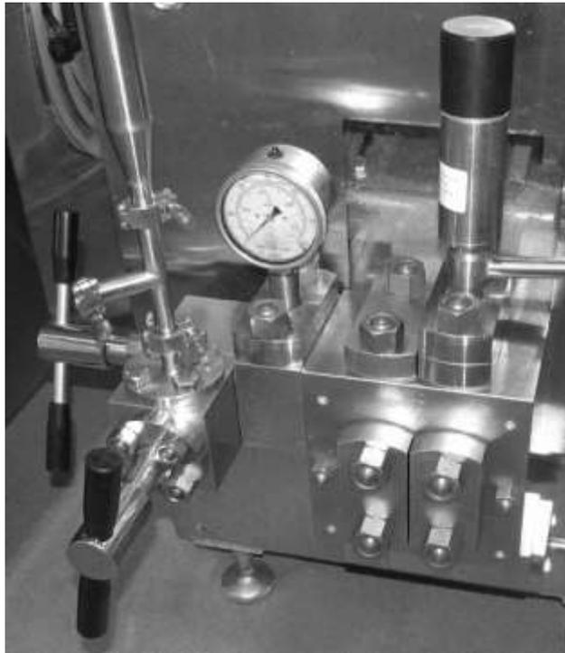
**The black handles on the left of this photo are used to adjust the openings of the valves on this two-stage homogenizer unit.**
