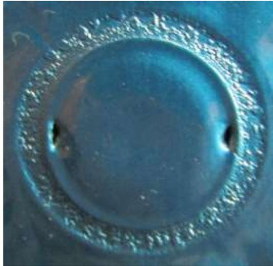
**This close-up photo shows the two openings in the degassing valve on a package of roast coffee.**
