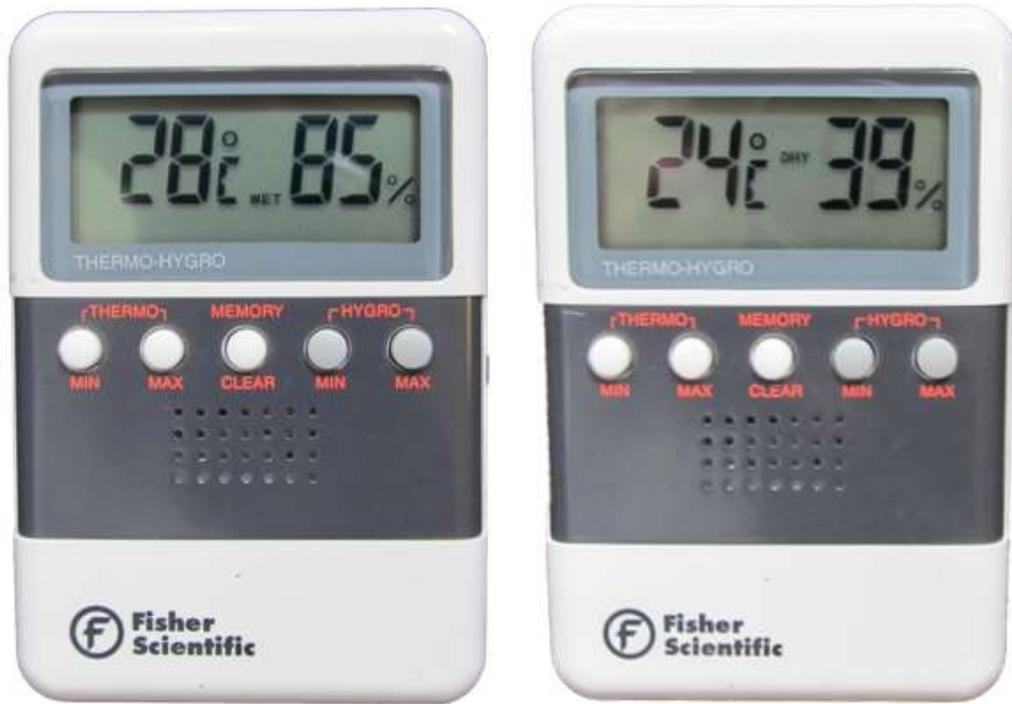
**These electronic thermometer / hygrometer devices show the temperature and relative humidity of air under two different sets of conditions.**
