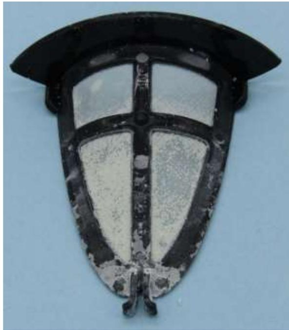
**Screen from a small kettle plugged with calcium carbonate particles.**
