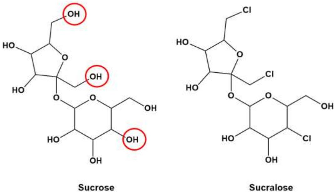
The three "OH" groups that are circled on the sucrose molecule on the left are replaced with chlorine atoms (Cl) to produce the Sucralose molecule on the right.
