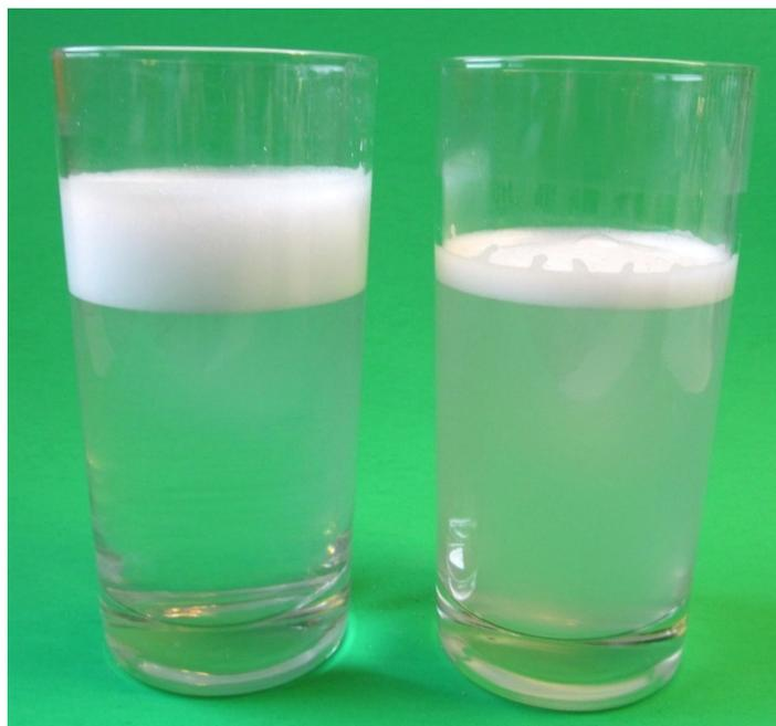
The glass on the left contains distilled water while the glass on the right contains water with added calcium ions. Note the difference in soap suds formation.
