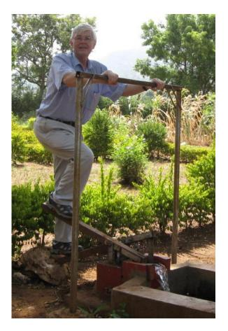
Using a Concrete Pedal Pump
