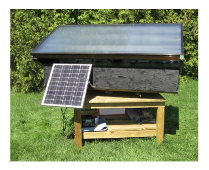
The "SolarFlex Dryer" with its heat collector on top to warm the incoming air. A solar panel for power is on the front. Product to be dried is placed on racks in the black drying chamber and the heated air is blown over it.
