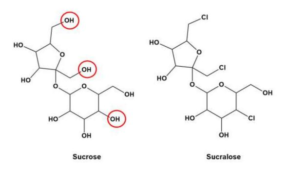
The three "OH" groups that are circled on the sucrose molecule on the left are replaced with chlorine atoms (CI) to produce the Sucralose molecule on the right.
