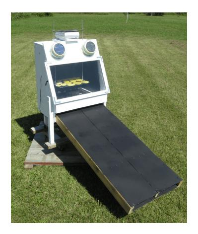
A small prototype solar dryer being used for research purposes. The large flat black surface is the heat collector.
