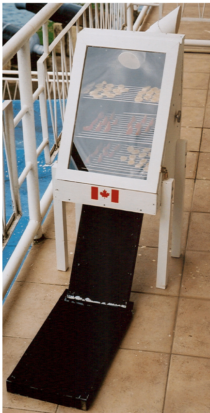
Figure 16: A solar dryer on location in Equatorial Guinea.
