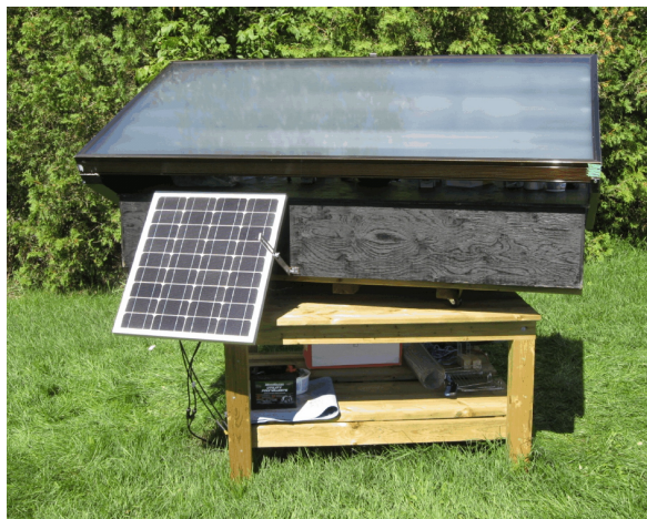
Figure 18: A modern solar dryer equipped with a solar panel to power fans
