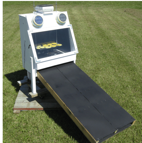
Figure 17: A solar dryer with solar-powered fans to circulate the air
