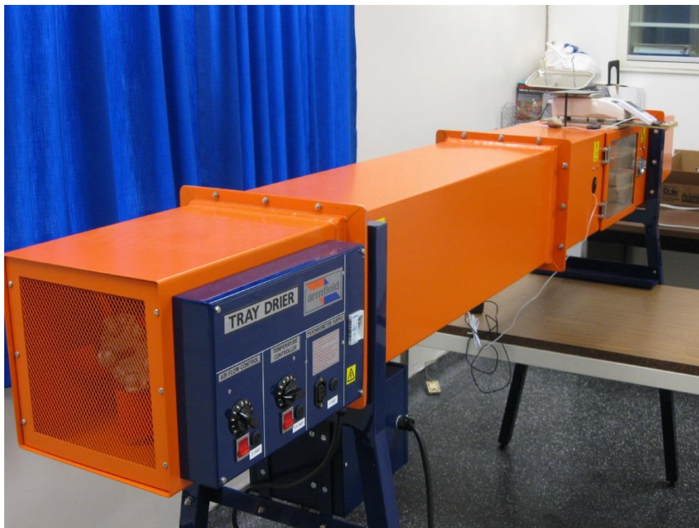
Figure 1: Armfield Laboratory-Scale Tray Dryer (Model UOP-8)
