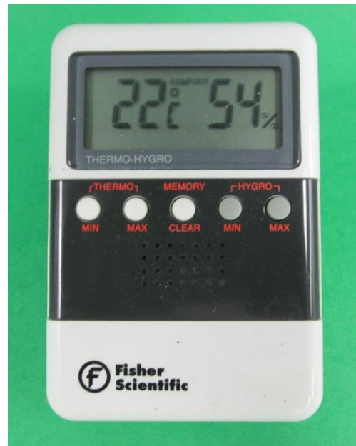
Figure 6: Digital thermometer and relative humidity indicator
