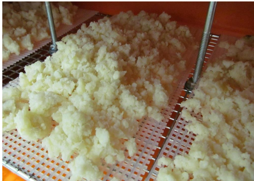
Wet mashed yams after being placed on plastic mesh in the dryer
