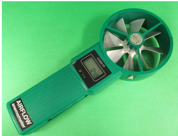
Figure 4: Hand-held vane anemometer for measuring air velocities
