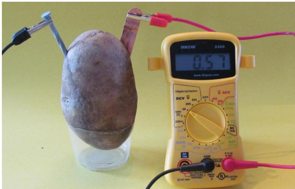
Potato battery showing voltage generated
