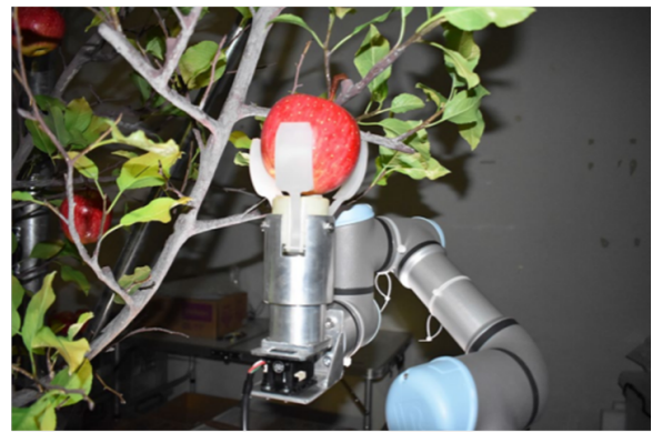
Figure 6. Left: example apple detection results based on deep learning model SSD. Right: apple harvesting based on UR3 robots. (Onishi et al., 2019)
